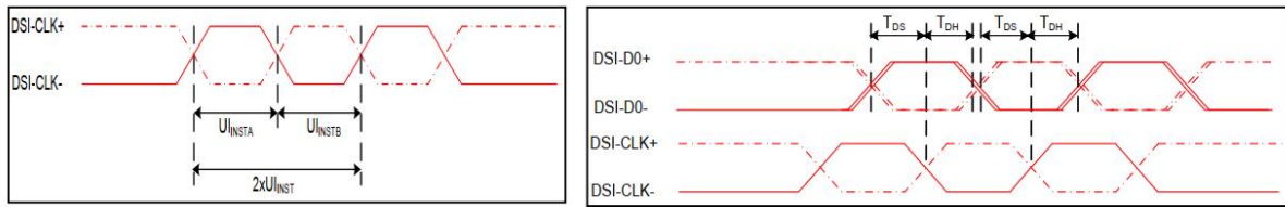
Figure 4 DSI clock channel timing
